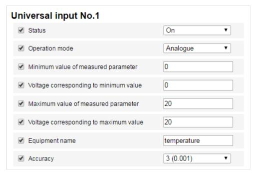
Measured Variable Minimum Value, set the minimum value for the variable measured by the sensor, defined in appropriate units. Voltage Associated With Minimum Value, set the voltage value that should be associated with the minimum value of the measured variable. Measured Variable Maximum Value, set the maximum value for the variable measured by the sensor, defined in appropriate units.
