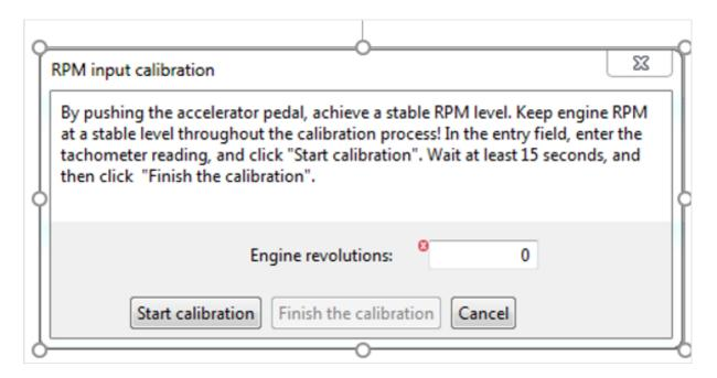
In the "Engine RPM", enter the number of engine revolutions according to the tachometer readings. Launch the calibration by clicking on the "Start Calibration" button. Wait for 15 seconds, and then click on the "Finish the calibration" button. The Omnicomm Configurator will determine the recalculation coefficient automatically. Save the recalculation coefficient in the Terminal by clicking on the "Record" button. Connect your tachometer to Smart Terminal according to the figure below:
