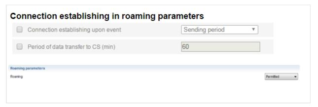
Roaming: Select one of the roaming options for your SIM card: 'Permitted', 'Disable', or 'According to the list'. To enable SIM card operation "According to the list in roaming" please enter MCC and MNC cellular networks to the Omnicomm Configurator.
