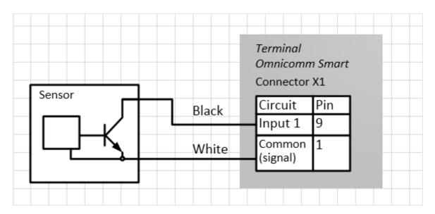
Connect contact sensors according to the figure below:
