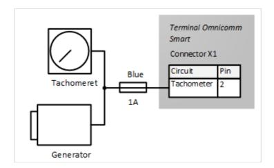
The tachometer's point of connection must be one in the vehicle's electrical network where the impulse signal frequency is proportional to the engine RPM rate.
