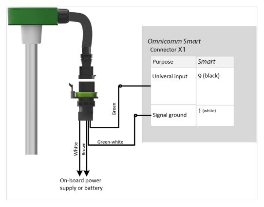
Omnicomm LLS-AF 20310 fuel level sensor shall be configured to deliver the frequency signal in the range from 30 to 1053 Hz.
