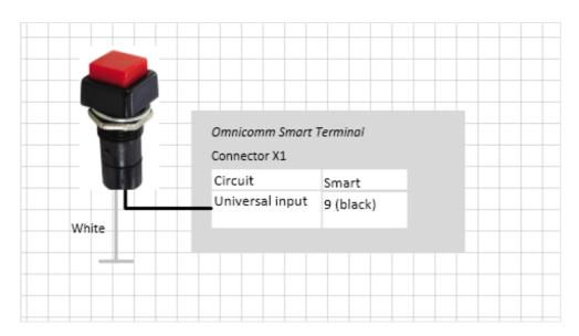
The panic button shall be installed on the vehicle's front panel, or anywhere inside the vehicle cabin that is convenient for use. Once you've chosen the installation place, drill a 12-mm hole, mount the button and secure it with a ring and a tab washer.
