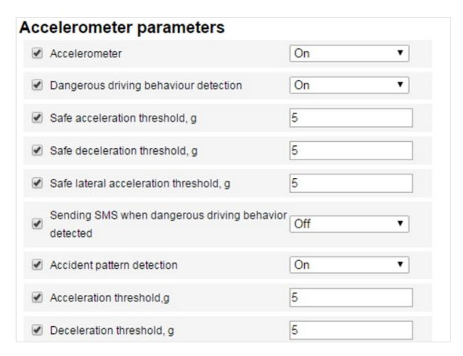
Accelerometer Parameters: Enable or disable these to switch the use of the accelerometer on or off in order to measure vehicle acceleration. "Dangerous driving detection" enable or disable to engage or disengage the evaluation of dangerous driving whenever preconfigured thresholds are exceeded.
