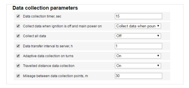
Collection Timer — set up the value for the polling period for the Terminal, its connected modules and external devices. The available value range is from 15 to 240 seconds.
