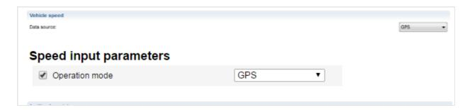
"Data source", select the data that should be used to record the events of ignition being switched on or off. Here are the available options: "Ignition key", this records the ignition being switched on or off by evaluating the position of the ignition key, given actual connection to the ignition key.
