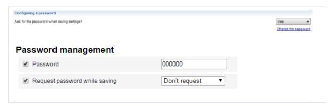
If you want to use a password for configuring the Terminal settings, select "Yes" as an answer to the "Ask for password when saving configurations?" field. Password, enter the password that will be used for access to settings configurations. The password must contain at least 8 characters.
