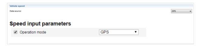
In "Data source" section please select what data should be used to calculate vehicle speed values. You can choose between GPS and CAN bus.
