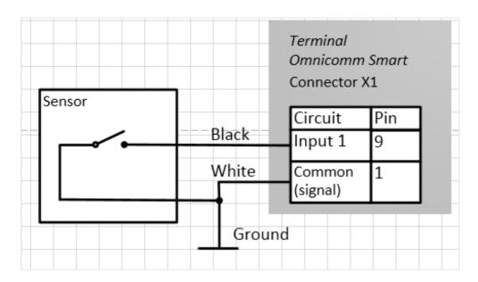
You can use standard factory equipment elements (such as on/off buttons, end switches/sensors that are activated by changes in temperature or pressure values, etc.) as contact sensors, or any additionally installed sensors. We recommend to first examine your options of connecting to a standard device or element, and only installing an additional sensor in case that this is not possible.
