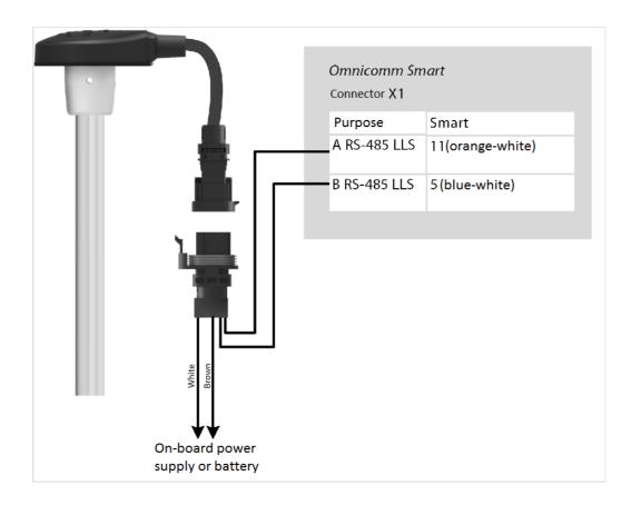
Connect the Omnicomm LLS 20310 fuel level sensor according to the figure below:
