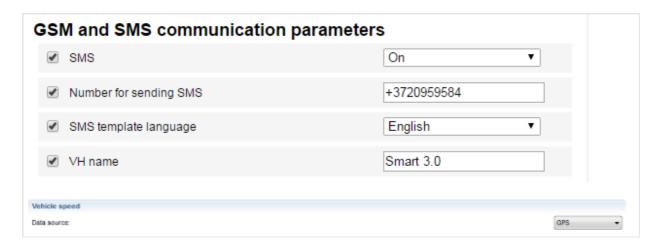
"SMS", switch on/switch off receipt of orders via SMS and sending of information
