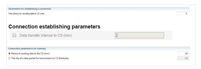
"Period of sending data to the CS", enter the number of minutes, upon expiry of which, the Terminal shall connect to the communication server when within the home network of your mobile network provider. The recommended value is 10 minutes.
